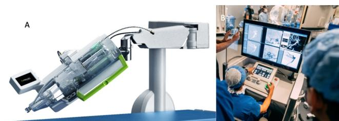
**Figure 2** CorPath GRX Robotic System. (A) Robotic arm with advanced cassette. (B) The set-up of the procedure. The primary neurointerventionalist was located in the corner of the angiography room in a radiation-shielded workstation. At bedside, the team consisted of the specialised robotic technologist and two neurointerventionalists who load the devices and control the perfused lines and hubs.
