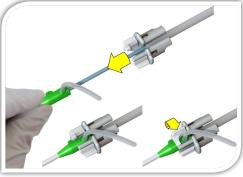
9. Turn lever on track clamp clockwise 180° into the "locked" position
