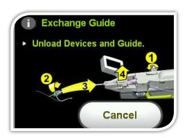
4. Turn track clamp counterclockwise into the "unlocked" position
